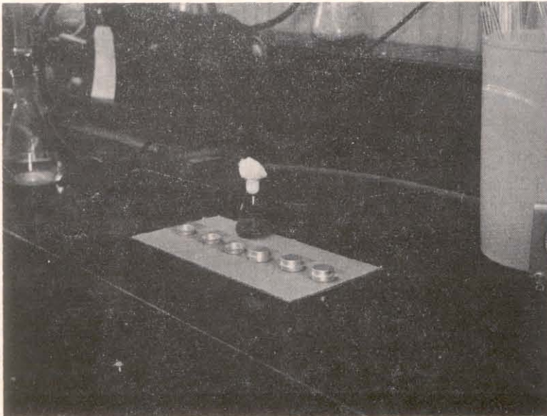
FIGURE 2.—Group of six coliform organism tests on carrying board. Three of the culture planchets have collection planchets positioned, but cover glasses have not yet been removed. Flask of labeled medium is displayed on carrying board for easy viewing.
