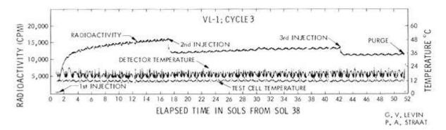
Figure 5. Complete VL1 cycle 3. A fresh sample was used in this active cycle. Data shows times of first, second, and third injections. [Reprinted from Levin, G.V. and Straat, P.A. (1977b) Life on Mar? The Viking Labeled Release Experiment. *Biosystems*, Vol. 9/2-3, pp165-174; with permission from Elsevier.]
