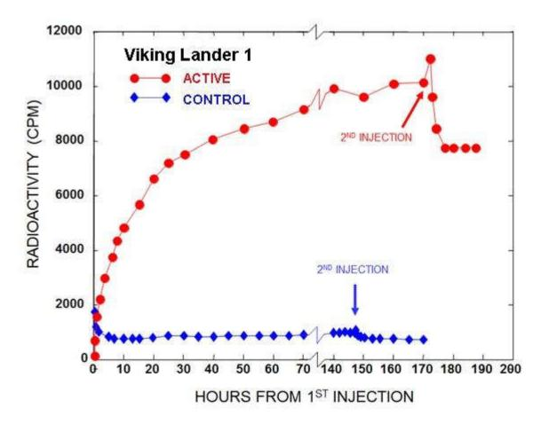
Figure 2. LR response to first and second nutrient injection in VL1 cycle 1 (active) and VL1 cycle 2 (160oC control). [Adapted from Levin and Straat, 1976b]
