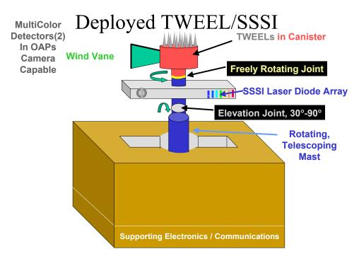
Figure 7. Deployed TWEEL/SSSI
