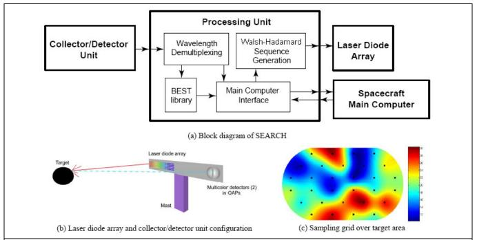
Figure 2. SSSI is composed of (a) the Laser Diode Array, the Collector Detector Unit, and the Processing Unit. The SSSI laser diode array (b) illuminates a target sample with an orthogonal Hadamard pulse sequence. Raster mapping at the black points (c) builds an image indicating what substances are present and their concentrations.
