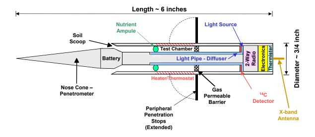
Note Sterilized canister contains multiple probes that are ejected away from spacecraft after landing.
