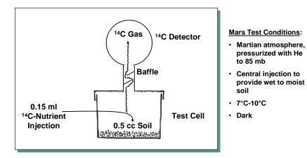
Fig. 2. Schematic of LR Instrument
