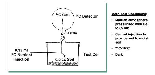
FIGURE 1. Schematic of the Viking Labeled Release Experiment
