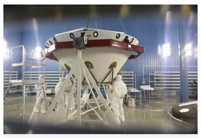
The descent module for ExoMars 2020 from the European Space Agency and Roscosmos will place the Rosalind Franklin rover on Mars, which could provide insights into the search for life on Mars. Image credit: Roscosmos
