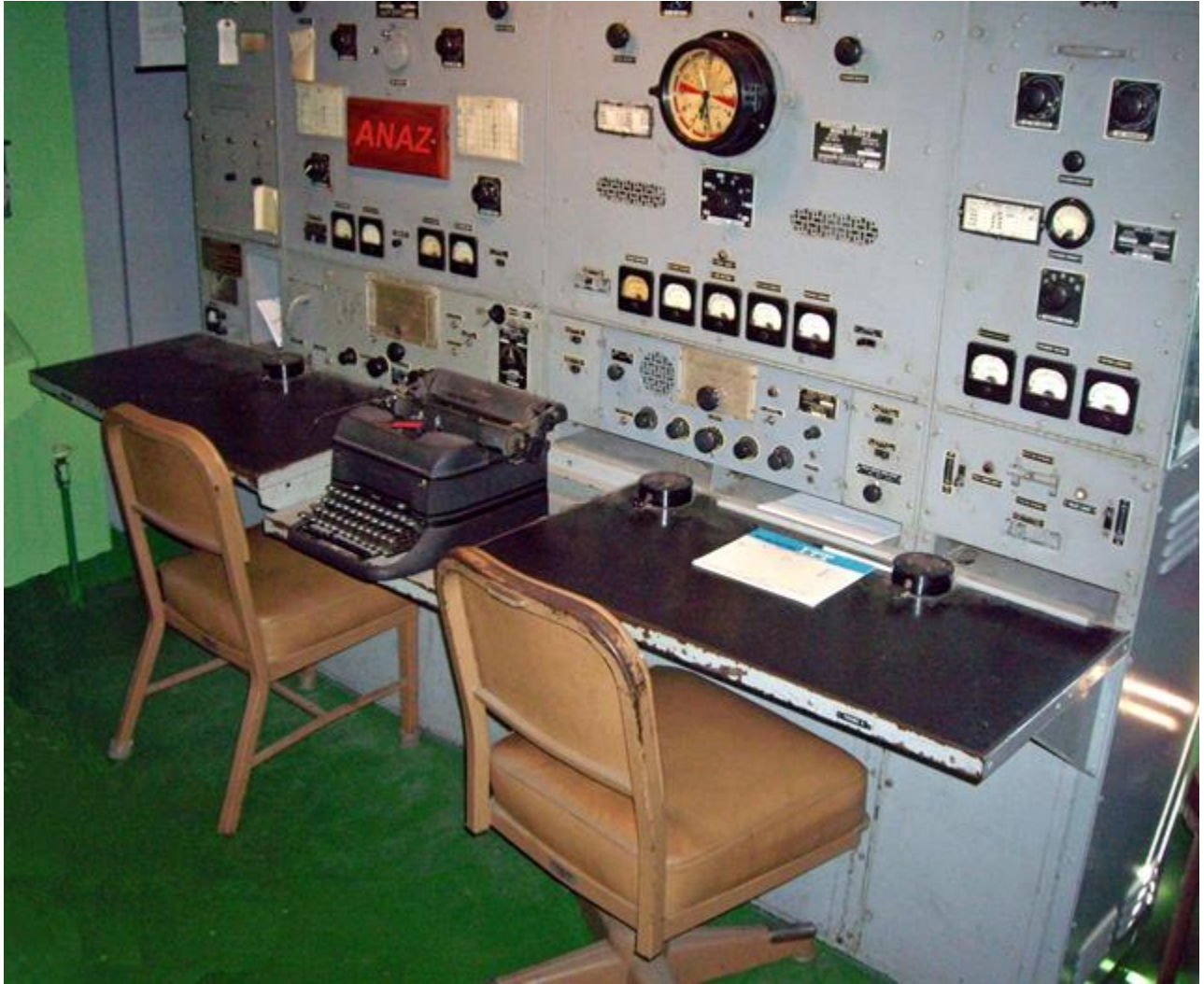
Radio operator console on a Victory Ship
