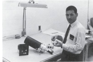
Fig. 4 Feasibility Model of Rocket-Borne Adenosinetriphosphate Assay Instrument
